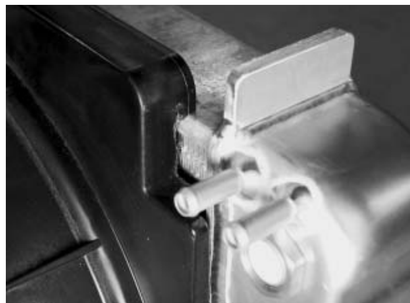
This photo shows how the notch fits over the larger core.
