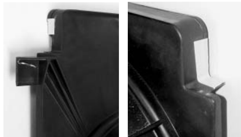
We applied a piece of masking tape to illustrate the shroud area that has to be trimmed out.
