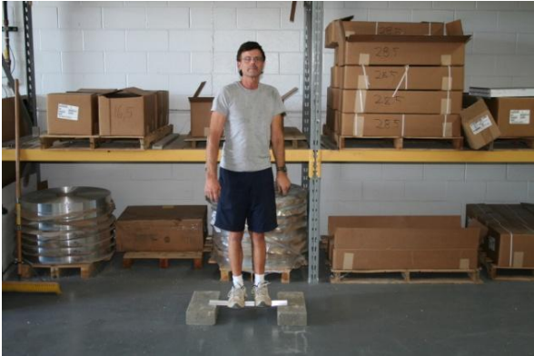
Extruded side channel (Holds 150 pound man)
